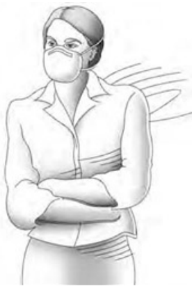
NIOSH-Certified ½ mask (N95) or Dust mask APF = 10 Needs to be fit tested
