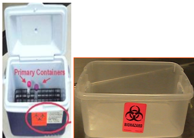
Figure 9: Example of Primary Container with Labeled Secondary Container (Princeton University, 2009)
