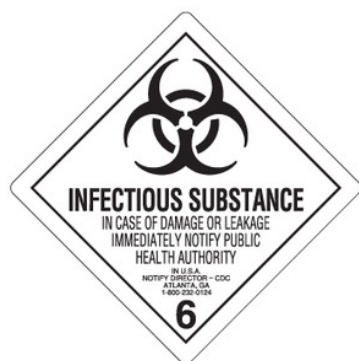
Figure 8: Example of DOT Infectious Substance Label. This label may be used in lieu of the "BIOHAZARD" label for shipped containers.
