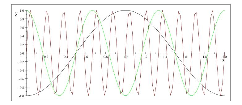
Let  $u_k = signal$  picked up at time kT. So  $u_6, u_{18}, u_{30}, ...$  will be 60 Hz signal. To cancel it, we use the min point: at the second max point  $u_{18}$ , we use the previous min point  $u_{12}$  to cancel it. Thus the filter  $y_k = u_k + u_{k-6}$ , or  $Y = (1 + z^{-6}) U$
