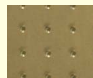
Object: Metal Optical Board with hole spacing 2.54 cm
